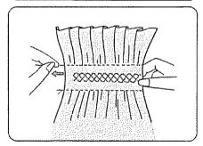
With the stitch length at "6", sew straight stitching lines 3/8" (1 cm) apart across the area to be smocked. Knot the threads along one edge. Pull the bobbin threads and distribute the gathers evenly. Secure the threads at the other end. Sew the decorative stitch between the gathering stitches. Pull out the gathering stitches.
